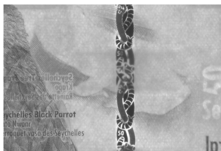
Transmitted infrared 860 nm, 5x. Security thread
