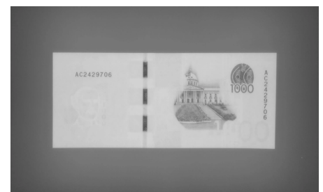
Incident infrared 950 nm, 1x. IR metamerism ink
