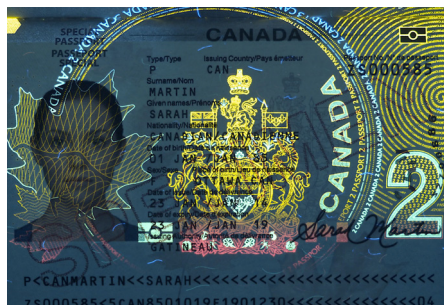
Ultraviolet 365 nm, 1.7x. Security fibers
