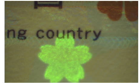
High-intensity infrared 950 nm, 15x. Anti-Stokes effect
