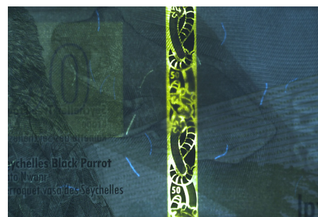
Transmitted ultraviolet 365 nm, 5x. Security thread
