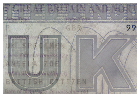
Diffused multi-position coaxial, 4.5x. Blind embossing
